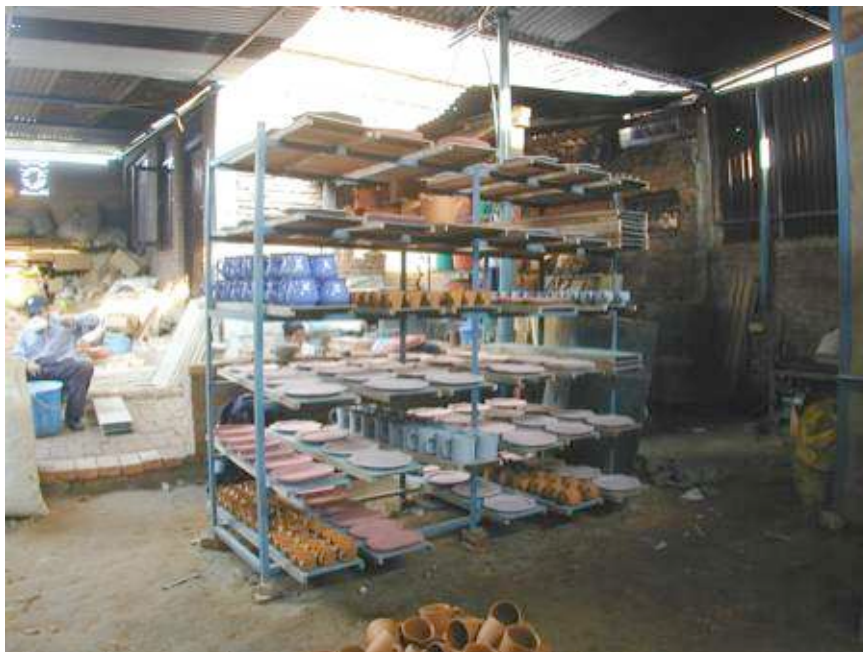
storage of glazed ceramics ready to fire
