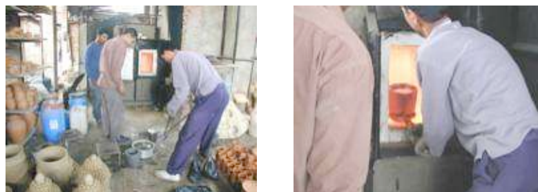
Shyam Shresta loads crush bowl with test frit
