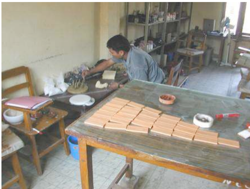
Sun Hari prepares triaxial tests with industrial glaze CG 231
